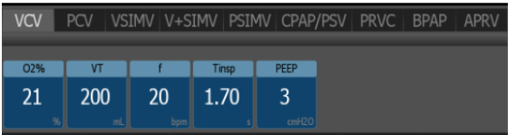
Figure 5-3. Ventilation Mode Control Settings
